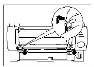
(7) Lift the tab to lock the side cutter into place.
